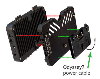
Place the EnduroPower bracket on the rear of the Odyssey7 . Secure the bracket with 1/4" flat head screw and tighten with Allen Wrench provided. Attach two 3mm flat head screws and secure with Phillips screwdriver.
